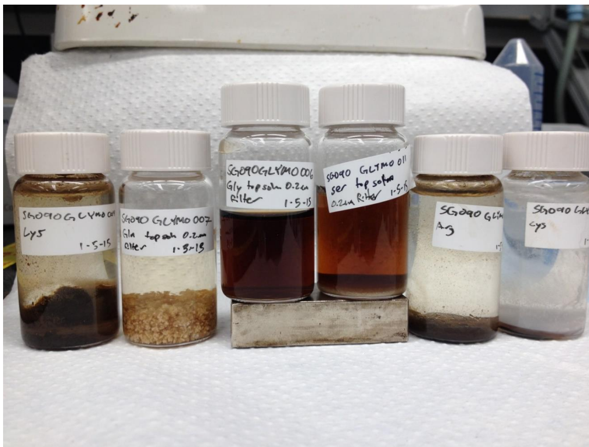
Figure 4.9. Visual aqueous stability assessment at pH=7.4 in presence of a magnet of several nucleophilic ligands used to open the GLYMO epoxy ring. Aqueous stability was indicated by a clear brown top solution as seen in Gly-FeOx and Ser-FeOx. From left to right: Lys-FeOx, Gln-FeOx, Gly-FeOx, Ser-FeOx, Arg-FeOx, and Cys-FeOx.
